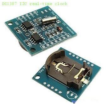
DS1307 I2C real time clock chip (RTC) 24C32 32K I2C EEPROM storage LIR2032 rechargeable lithium battery with charging circuit Solve the read/write problem of the DS1307 with spare battery. After fully charged, it can provide one-year DS1307 timing. Compact design, 27mm\*28mm\*8.4mm in size Extract DS1307 clock pin, providing clock signal for the microcontroller
